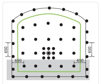
RECOMMENDED UNDERGROUND DEVELOPMENT HEADING Tie in 5g Detonating cord to be < 500mm from perimeter holes (shown in green)
