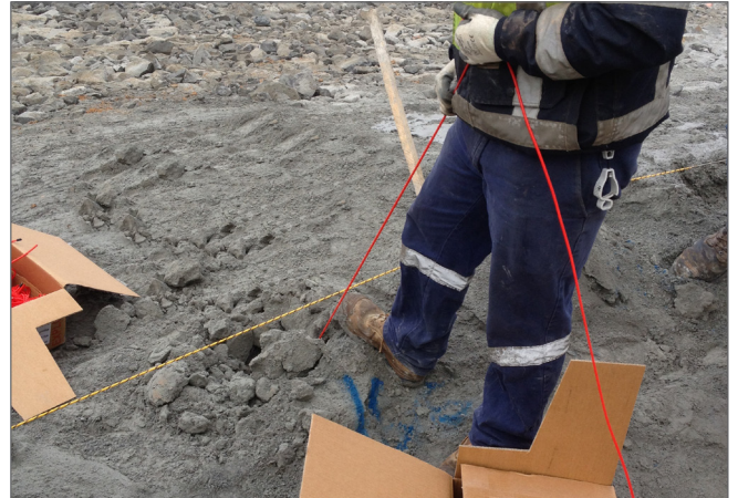
4. Lower MEGASPLIT® product down the bore hole in a controlled manner.
