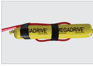
4. When using detonator cord, thread the cord carefully through at least two cross-cutting holes made with the skewer, attach the cord to the cartridge with electrical tape (starting and finishing at the top) before securing the cord to itself (by knot or tape).
