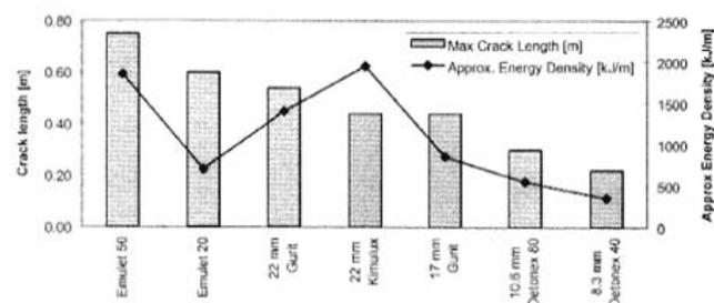
FIGURE 14. Maximum Crack Length measured for various explosives (and decoupling ratios), all in 38mm holes and calculated approximate linear energy densities for the explosives used (crack data from Ouchterlony 1995; and explosive energies taken from Persson , et al 1993).
