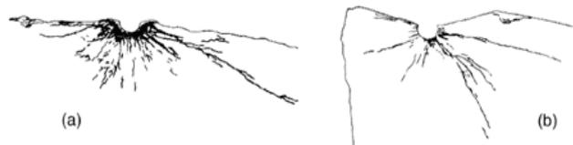
FIGURE 17. Comparison of crack patterns for two explosive charging configurations with similar Decoupling ratios (after Olsson , 1996). (Note different depths of damage; also not necessarily to scale.)
