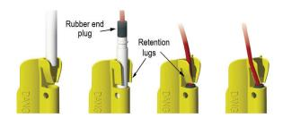
3. Insert the Mighty Atom's loading guide onto the end of the ANFO hose.
