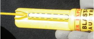
2. Clip the shock-tube into the retention lug
