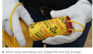
4. When using detonating cord, thread the cord fully through both tunnels (starting and finishing at the red capped top) before securing the cord to itself (by knot or tape).
