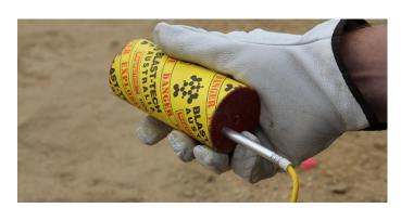
When using detonators, begin by inserting the detonator into the larger diameter (cord) tunnel in the red cap at the top of the booster.
