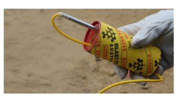
3. Rotate the detonator 180° and reinsert into the empty detonator capwell.
