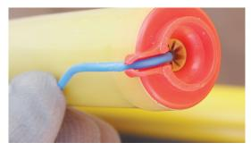
**3.** Gently pull the detonator signal tube around and press it into the signal tube retention clasp.
