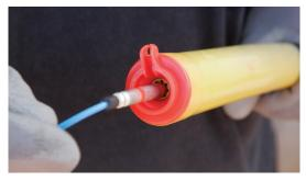
**1.**Insert the detonator into the capwell that is fitted to the flared end (primer end) of the coil.
