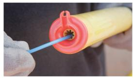
2. Ensure the detonator is fully inserted into the capwell.
